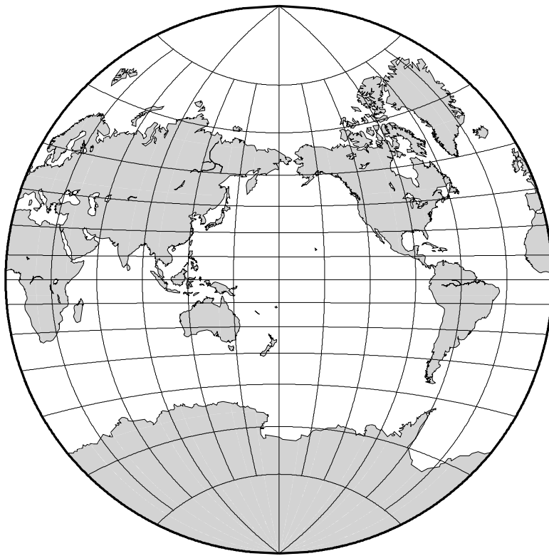
Figure 6.33: World map using the Van der Grinten projection.
