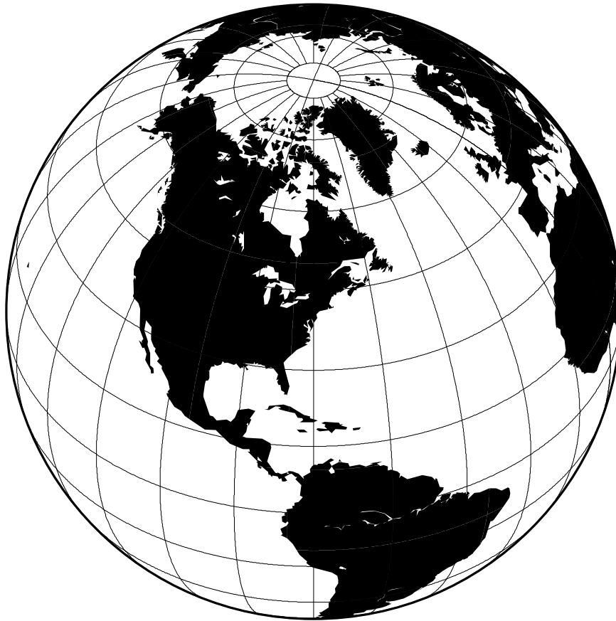
Figure 6.12: Hemisphere map using the Orthographic projection.
